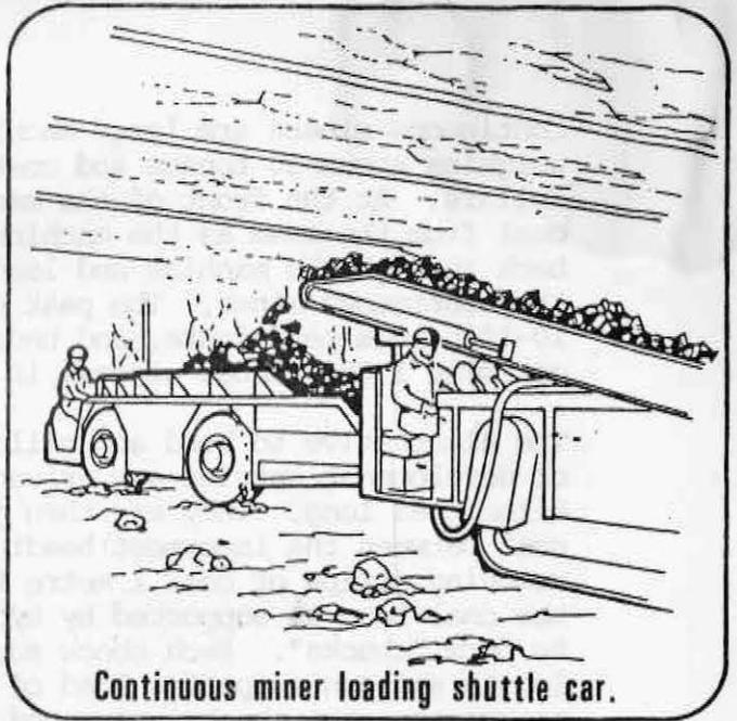
Continuous miner loading shuttle car.
