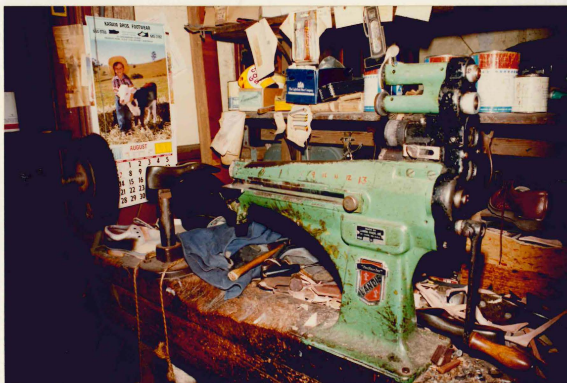
Cutting machine, with 2 cutters and a skiver on it. The skiver trims around the finished shoe.
